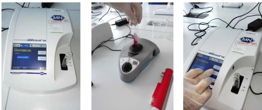
Fig. 9.9. Subsequent activities while performing the exercise (from the left: placing the sample in the measurement chamber; mixing the solution on the stirrer type VORTEX; reading the absorbance of the sample)
